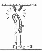
Mechanics: F2 increases compared to F1 giving a tendency to pull the knot past climbing rope elongate more than the the sling. Since this will not occur because of the restriction offered by the sling the slings remain intact.
